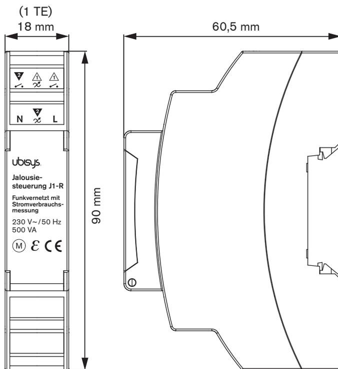
Figure 2: Rail-mount ZigBee Shutter Control J1-R – Dimensions
