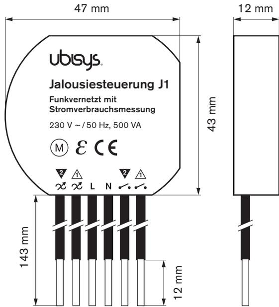
Figure 1: Flush-mount In-wall ZigBee Shutter Control J1 – Dimensions
